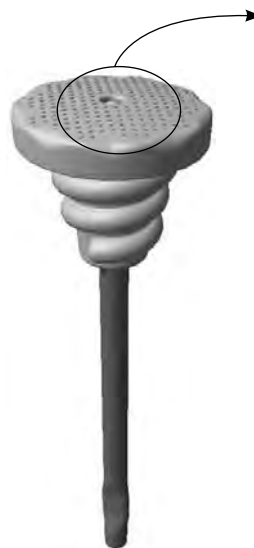
Detail B Step 5 Attach the stationary button to the bounce button post.
